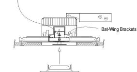
Flanged Trim installs into fixture housing by integral leaf springs.
