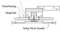
Wing Nuts for fine leveling adjustments
