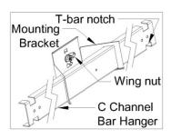
Step slots for ceiling thickness adjustments.
